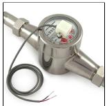
Flow sensors with 3 wires and runs on 5V can also be used with OpenSprinkler. In this 0 case, insert the ground wire (typically black colored) GND, 5V wire (typically red colored) to VIN, and the sensor wire (typically yellow) to SN1.
